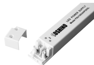
PC casing, screw terminals (input 2x0.75mm 2 output 2x1.0mm 2 ) with screw-down covers
